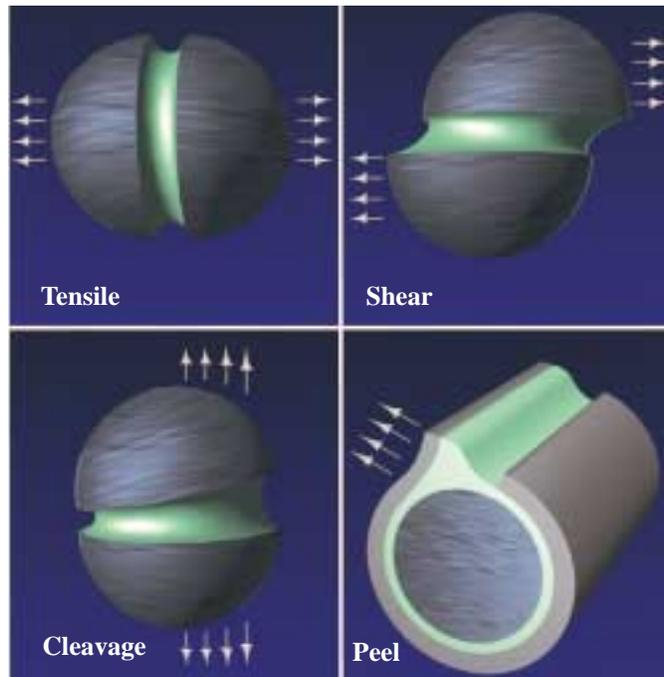
**Tensile** is pull exerted equally over the entire joint. Pull direction is straight and away from the adhesive bond.
